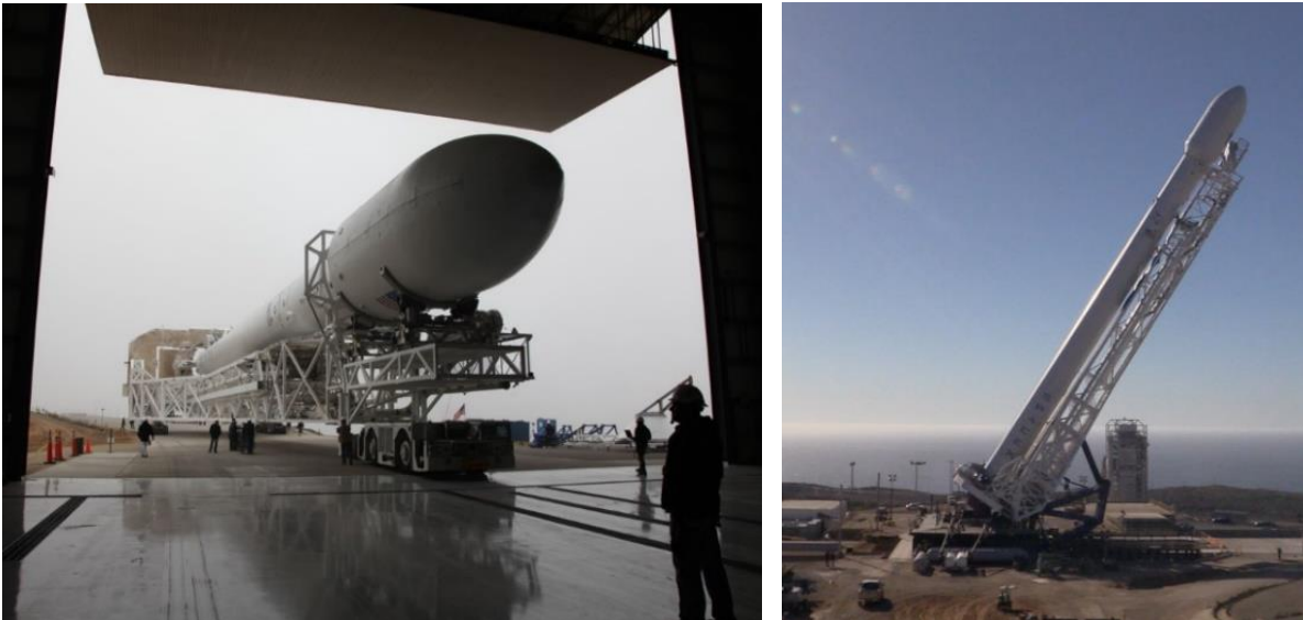
Figure 10-10: Launch Vehicle Rollout and Erection
