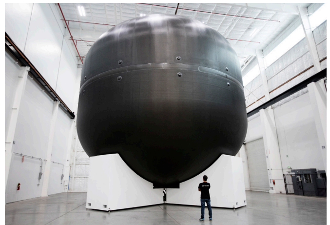
Fig.1. Deep cryo liquid oxygen tank developed by SpaceX
